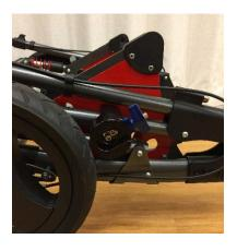
The images above shows a Daessy Mount using UFC1000IPMOD Narrow Frame Clamp Inner Piece 1" Round UFC1000IPMOD Narrow Frame Clamp Piece 1" Round with a RFCR.
