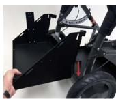
6) Hang the Rear tray section on the rear crossbar ON TOP OF THE MIDDLE SECTION. Press down firmly on the crossbar to make sure the Top section seats securely and evenly OVER the Middle section.
