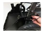
7) Locate the top / front slot next to the "Z" shaped padded flange. Slide the Velcro "D" ring strap thru slot making sure to leave the ring on the inside of the tray.
